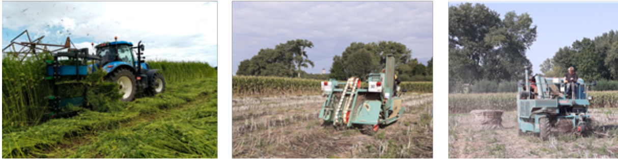
Fig. 1. Automated harvesting (left), turning (mid) and baling (right) of hemp for the flax processing line (summer 2020, Bottelare, Belgium).
