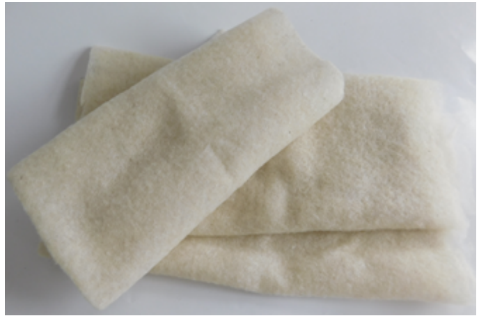
Fig. 3. Needled nonwoven made of wool and poultry feathers.
