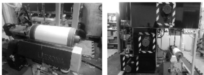
Figure 2. Extrusion of Functionalized PLA Multifilaments
