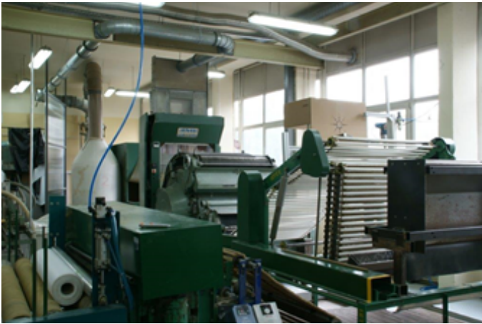
Fig. 2. Experimental line for the production of needle punched nonwovens.
