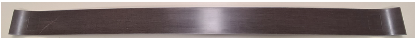
Fig.1 Leaf spring element of a bogie of a narrow-gauge railway made from the developed flax yarn (quasi-UD fabric) and an epoxy matrix (length 1170 mm, width 90 mm).
