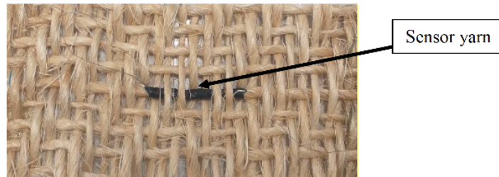
Fig. 1: Yarn strain sensor inserted inside the 2D fabrics
