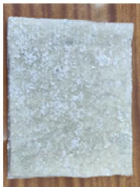
Fig.2 Nonwoven fabric with the addition of cotton fibers from the production of bedding
