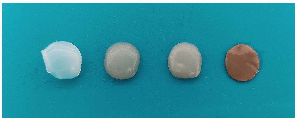
Fig. 2 BNC membranes embedded with lignin. From left to right: BNC, lignin 0.05M NaOH, lignin 0.1M NaOH and lignin.
