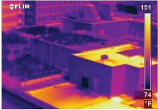
Temperature differences between a green roof and a conventional roof
