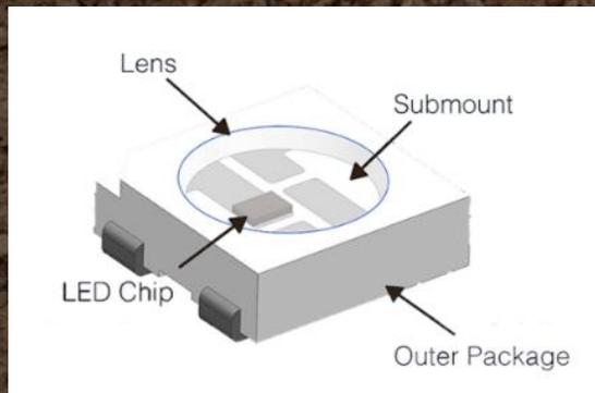
Figure 2: UV-C LED Structure [1]
