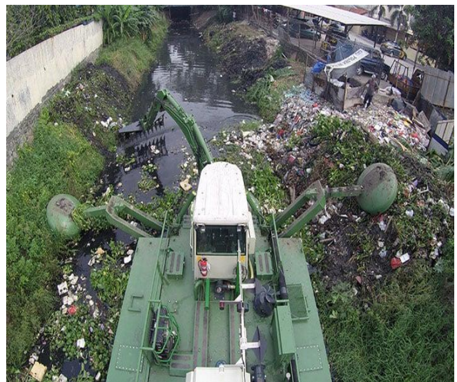
Fig[5]. The Multi-Purpose Amphibious Dredger working [8]
