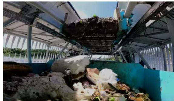
4. **“Dumpsters:** The Interceptor can store up to 50m<sup>3</sup> of trash before needing to be emptied. This means it is capable of operating even in the most polluted rivers all over the world.”
