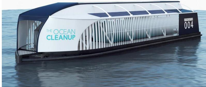
It collects energy by means of solar panels and store energy in lithium batteries. These batteries allow you to operate continuously day and night autonomously. Intelligent on-board software monitors system performance, energy use and component status.
