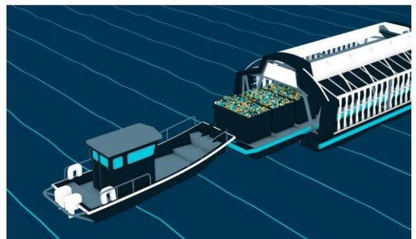
5. **“Empty and recycle:** When the interceptor is almost full, it automatically sends a text message to the local operators to come and collect the waste. Operators then remove the barge, bring it to the side of the river, empty the dumpsters, send off the debris to local waste management facilities, and return the barge back into the Interceptor.”
