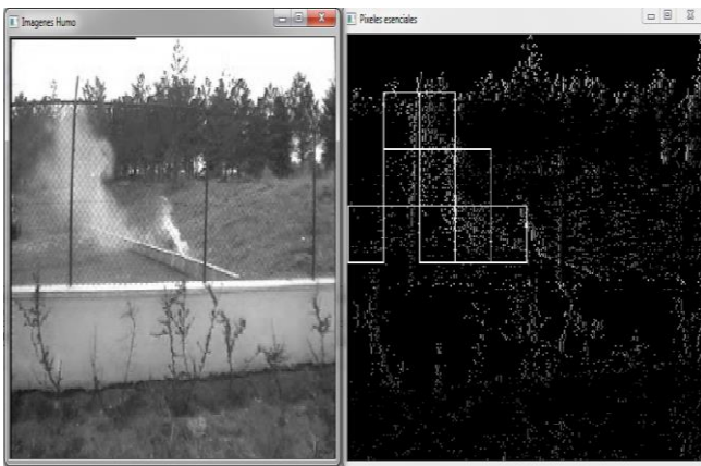
Fig. 8. Marking on a video of "Smoke" regions in real time. Resolution 320x240 pixels. Capture of the program developed in C, platform Netbeans.
