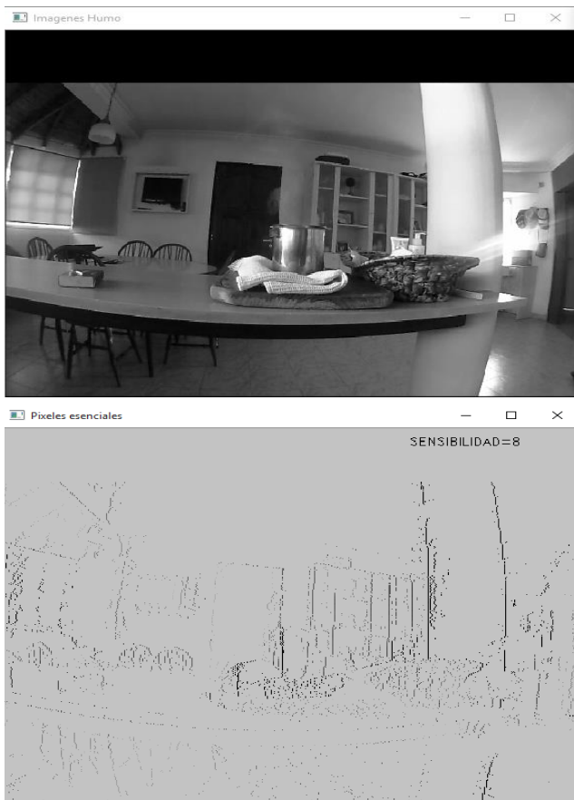
Fig.3. Indoor scene and essential pixels for interpolation error of 5%. Image of 640 x 480 pixels, gray levels.
