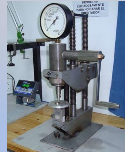
Adhesion VDI 3198 Rockwell C Indentation
