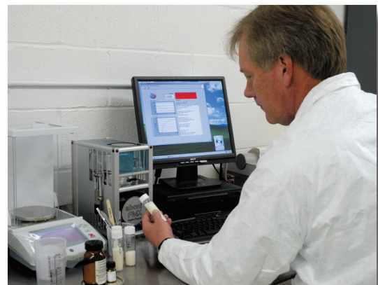
Measuring moisture content of material samples
