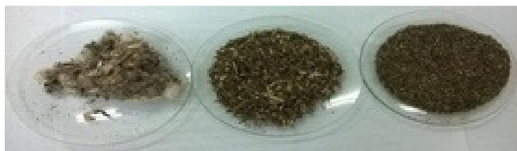
Figure 1. Original and two different particle size samples of waste cotton fibrils
