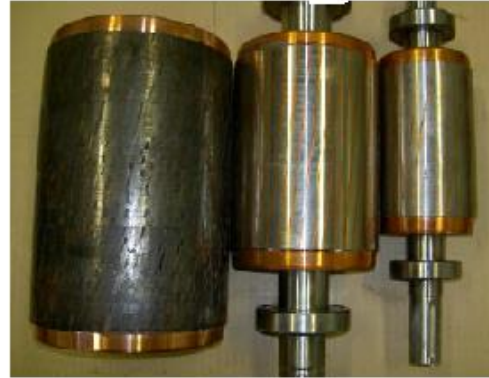
Fig. 3 – View of copper rotors for the considered motors
