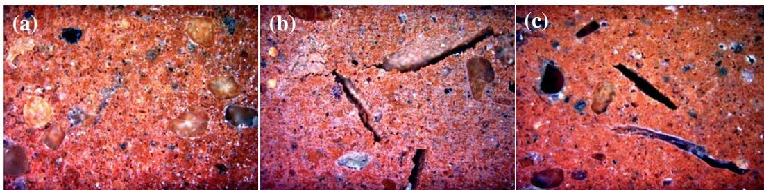
Figure 5: Optical microphotographs of the samples (a) CCB, (b) RHB, (c) SSB. Magnification: 50X.
