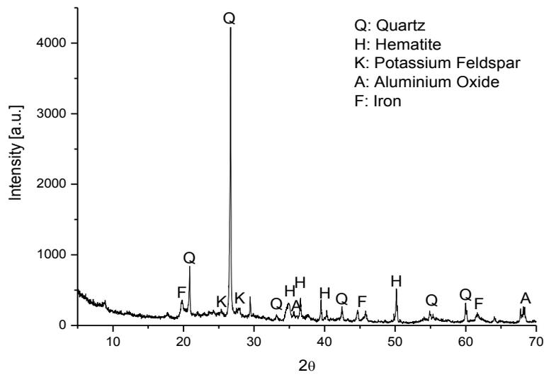
Figure 2: XRD pattern of commercial clay.
