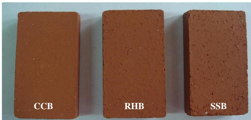
Figure 4: Macroscopic appearance of the obtained bricks.
