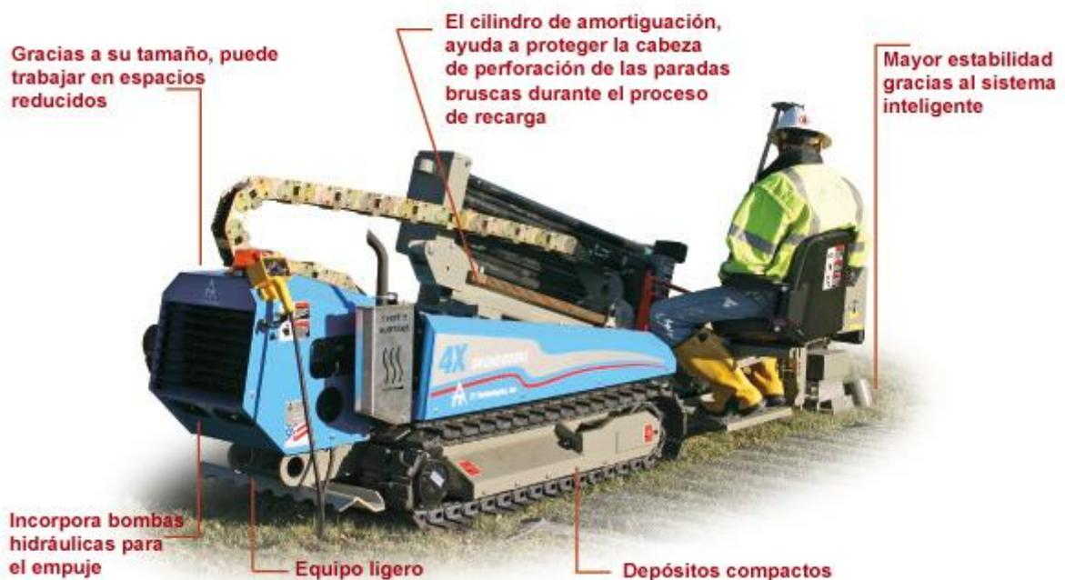
Figura N°29: Grundodrill 4X
