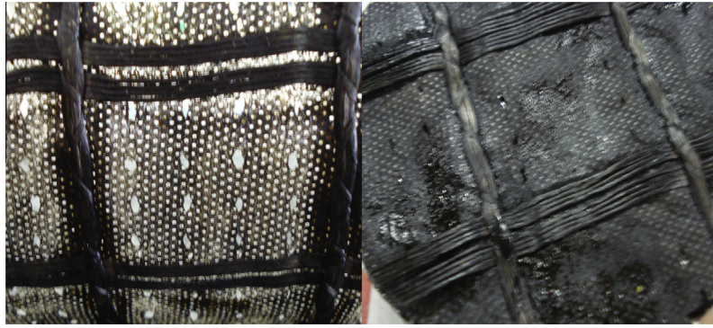
Fig. 1. Commercial geosynthetic (left) and impregnated with modified asphalt emulsion (right).
