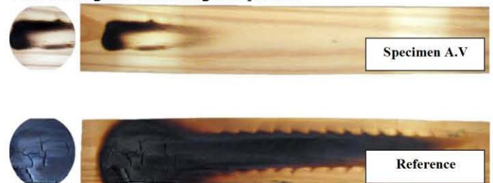
Fig 2. Flame Spread in Two-Foot Tunnel
