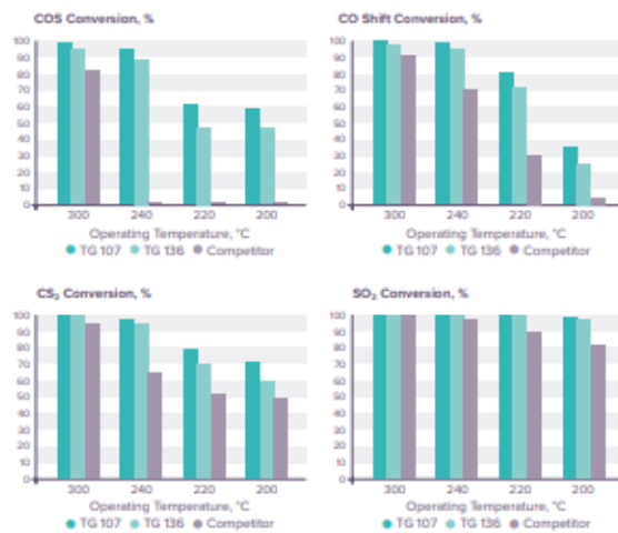
↑ Figure 2: Comparative tests with SulShine™ TG 107 and SulShine™ TG 136
