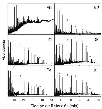
**Figura 13.** TICs de los crudos AN, BS, CI, DB, EA y FI. 1: decano (n-C<sub>10</sub>), 2: tridecano (n-C<sub>13</sub>), 3: heptadecano (n-C<sub>17</sub>), 4: docosano (n-C<sub>22</sub>), 5: pentacosano (n-C<sub>25</sub>), 6: octacosano (n-C<sub>28</sub>).
