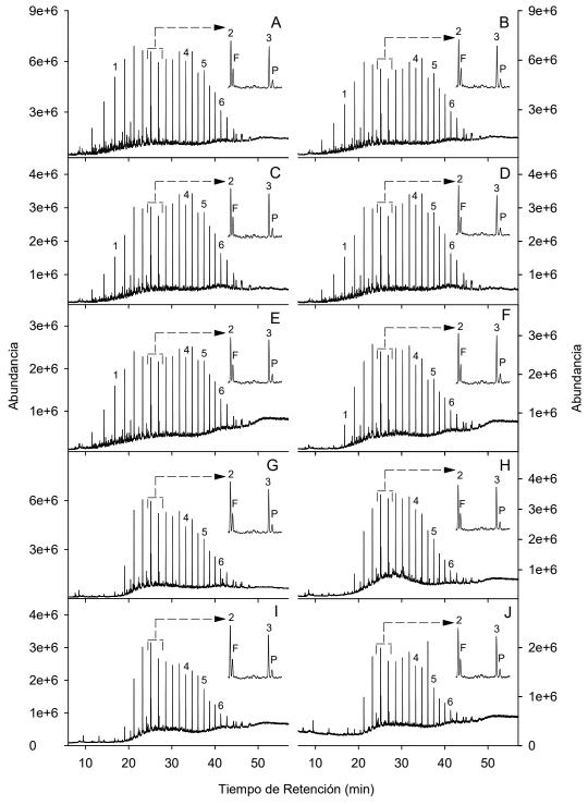
**Figura 22.** TICs del crudo AS extraído de suelo a los tiempos T0 (A) a T9 (J). 1: tridecano (n- $C_{13}$ ), 2: heptadecano (n- $C_{17}$ ), 3: octadecano (n- $C_{18}$ ), 4: docosano (n- $C_{22}$ ), 5: pentacosano (n- $C_{25}$ ), 6: octacosano (n- $C_{28}$ ), P: pristano, F: fitano.
