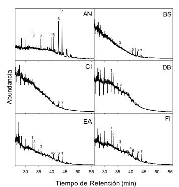
**Figura 14.** Fragmentogramas (m/z = 191) de los crudos AN, BS, CI, DB, EA y FI. 1: terpano tricíclico  $C_{23}$  ( $T_{23}$ ), 2: terpano tricíclico  $C_{24}$  ( $T_{24}$ ), 3: terpano tricíclico  $C_{26}$  ( $T_{26}$ ), 4: trisnorneohopano (Ts), 5: trisnorhopano (Tm), 6: norhopano  $C_{29}$  ( $H_{29}$ ), 7: hopano  $C_{30}$  ( $H_{30}$ ).
