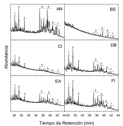
**Figura 15.** Fragmentogramas (m/z = 217) de los crudos AN, BS, CI, DB, EA y FI. 1: esterano  $C_{20}$  ( $S_{20}$ ), 2: esterano  $C_{21}$  ( $S_{21}$ ), 3: esterano  $C_{22}$  ( $S_{22}$ ), 4: diasteranos  $C_{27}$  ( $D_{27}$ ). 5: colestanos ( $S_{27}$ ), 6: ergostanos ( $S_{28}$ ), 7: estigmastanos ( $S_{29}$ ).
